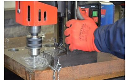
Drilling capacity up to 16 mm (0.63")
