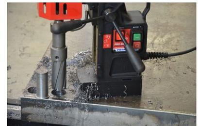
Milling capacity up to 55 mm (2.17")
