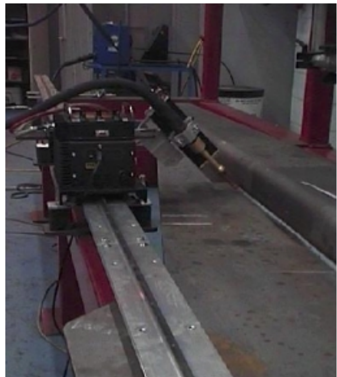
LASER-BUG in flat fillet welding.
