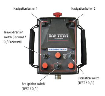
F1, F2, F3 - Rotary parameter/function setting knobs
